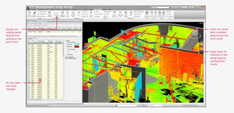
Leica CloudWorx for Revit is a breakthrough plug-in for efficiently using rich as-built point cloud data, captured by laser scanners, directly within Revit for better BIM modelling of existing buildings. This is useful for a wide range of BIM activities including retrofit design, construction and operations, and lifecycle asset management of the building. It provides a virtual visit to the site within Revit with a complete view of the captured reality.
