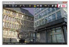
The easy to use JetStream Viewer connects to ProjectVault for 3D navigation (with support for 3D mouse), visualisation, measurement, image and video screen capture, quick limit boxes, and access to saved UCS' and limit boxes/slices.
