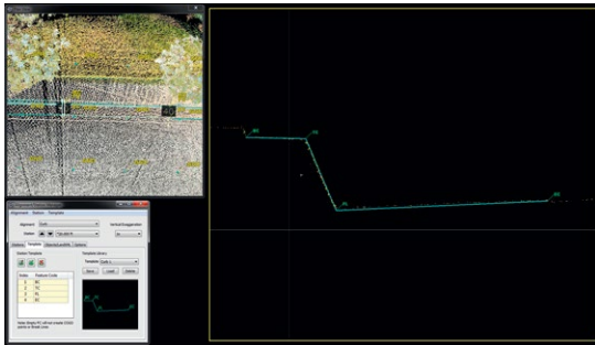
All new Alignment/Station Manager with a secondary Plan View window allows for easy creation of breakline from feature coded templates.
