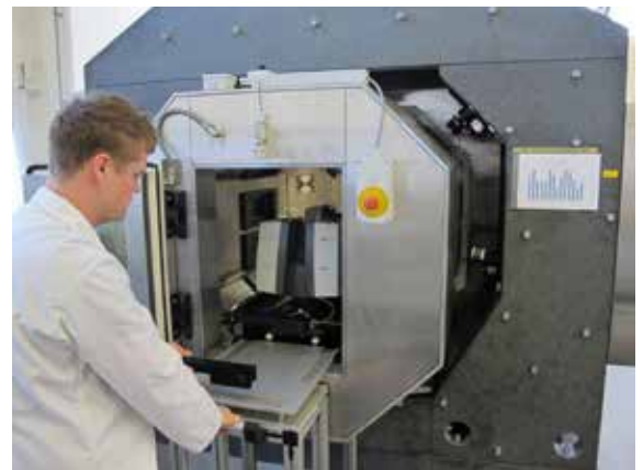
Figure 14: A Leica ScanStation P40 being loaded into the ATEC Rig.
