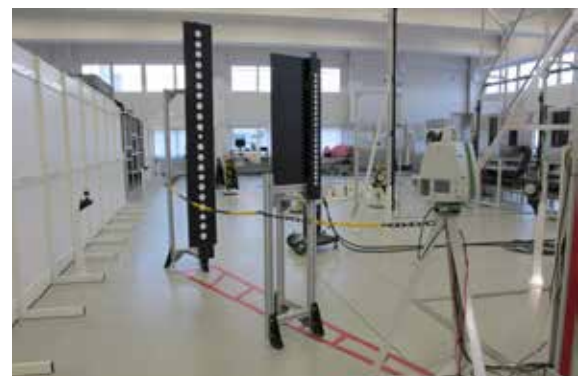
Figure 19: A view of the camera calibration stand. Two sets of targets are placed in front of the scanner and are both imaged and scanned.
