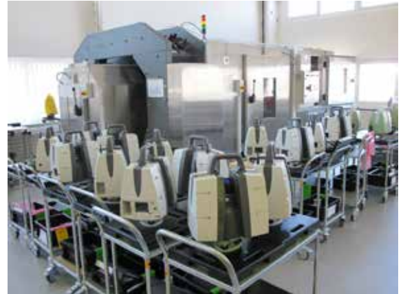
Figure 13: A collection of P40 scanners waiting for their turn on the ATEC Calibration Rig. To the human eye, they are perfectly identical, but the human eye is not designed to discern microns. To the Antipodal Telescope Environmental Chamber (ATEC), they are all as uniquely different as human fingerprints.
