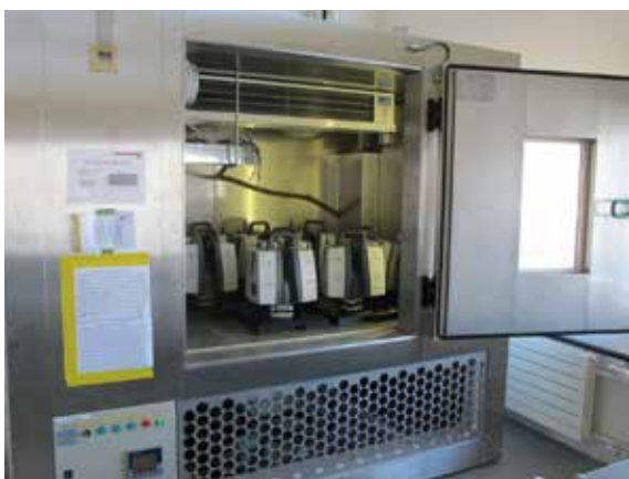
Figure 12: Environmental chamber for thermally cycling P and C series laser scanners. This station is called ESS, or Environmental Stress Screening.
