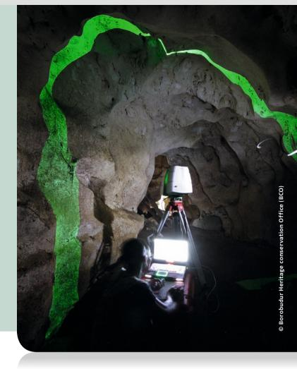
ScanStation C10 would serve as a reference point, helping to monitor Borobudur for any occurring changes caused by regional property development. Another task requiring use of the laser scanner was to assess the stability of the building site itself and also of threatening slope inclinations of the complex's surrounding hills, which could change at any time due to natural disasters.
