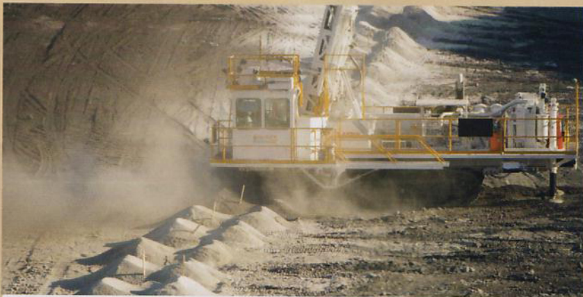
Leica's DrillNav Plus guides the drill and manages its operation.
