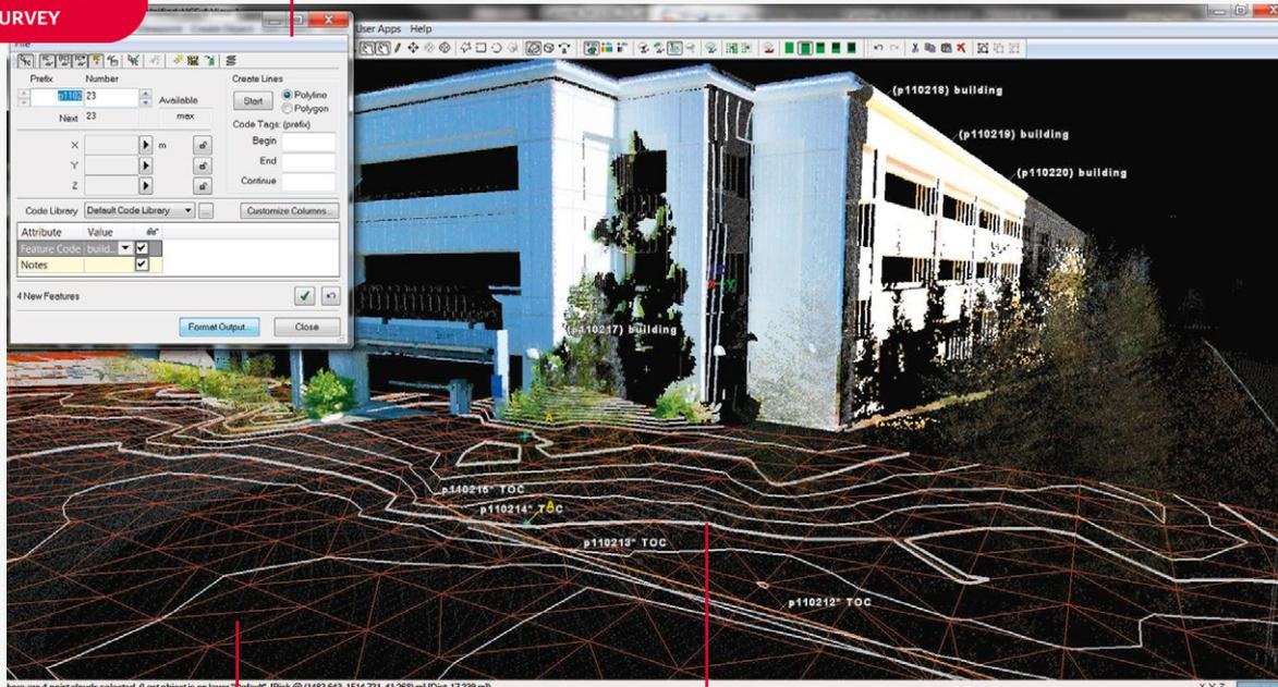
Automatic TIN mesh at any grid spacing
