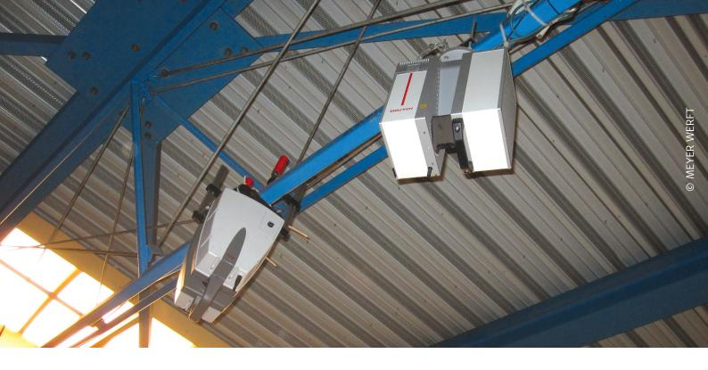
stage before prefabrication installations. We've also met more advanced standardisation requirements with 3D laser scanning, such as structure analysis, reverse engineering and volume determinations throughout the ship building process. In addition to geometric surveying for construction monitoring, the data provides documentation for warranty needs.
