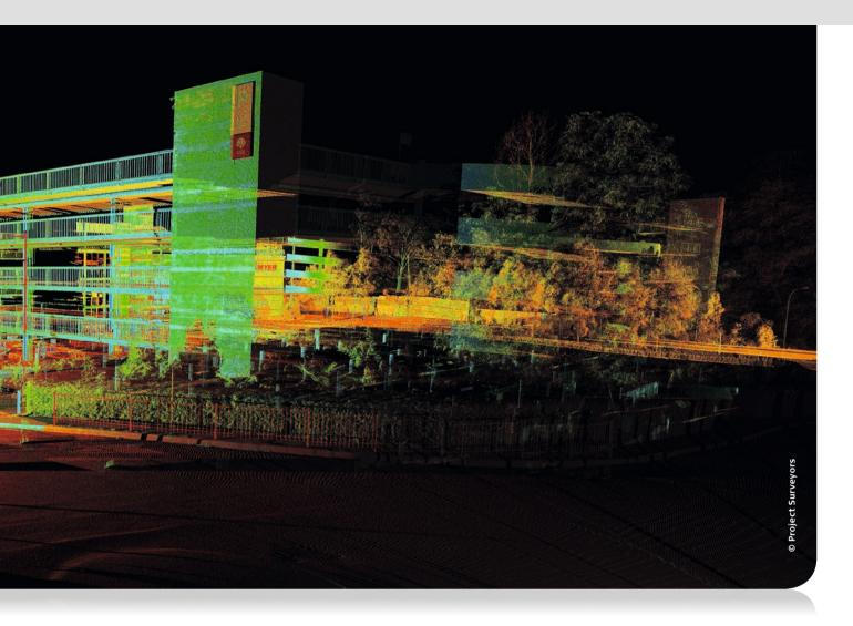
The Leica ScanStation C10 was used for the external facades and inside for large structures, such as the parking garages, due to its long-range capability. Inside, the Leica ScanStation P20 was used for its quality of producing fast reliable data at low resolution.
