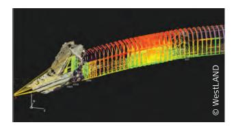
Railroad for use with double stacked trains, and 17 tunnels will have to be surveyed for clearance analysis and possible grading and track redesign. WestLAND saw the scan of one tunnel as basically a marketing investment and offered to scan one of the smaller tunnels, No. 15, which was only 91.4 metres long. It was the first project to make use of the MultiStation and it went very well.
