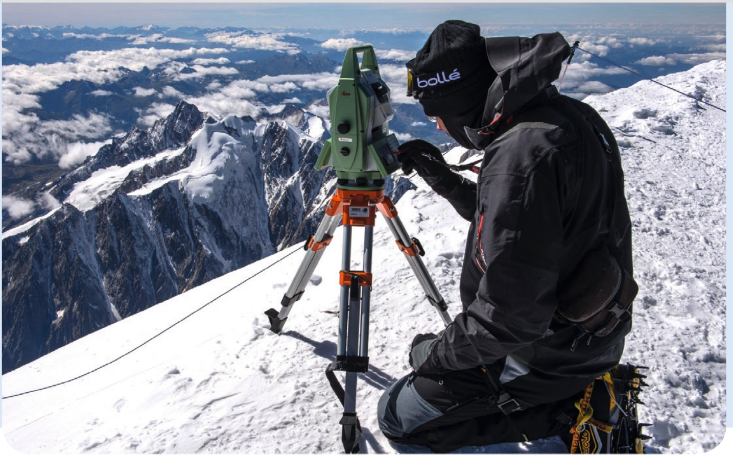
■ Setting up the MS50 MultiStation on the top of Mont Blanc.
