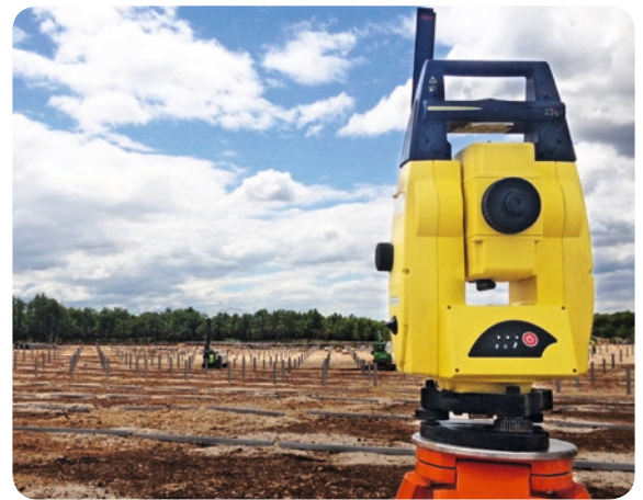
■ Post stake out using Leica iCON robot 50
