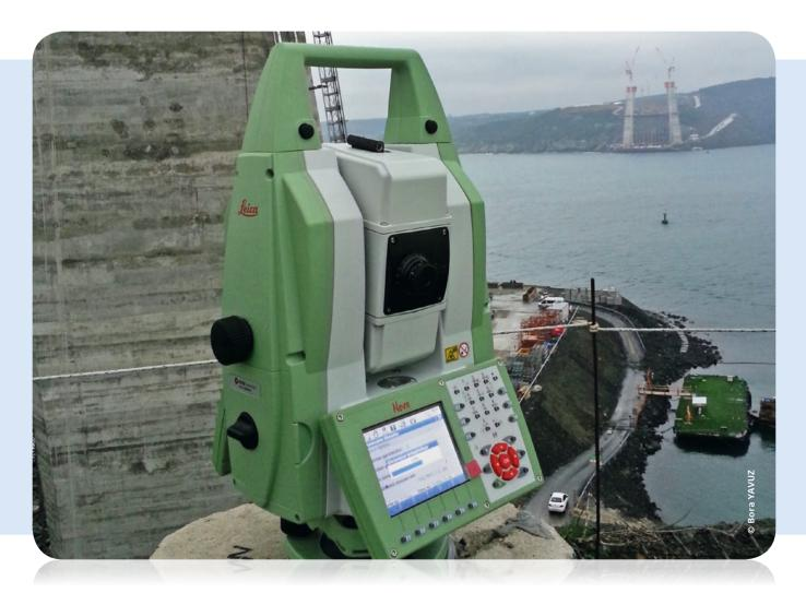
In addition, vertical alignments of the pylons were checked using several Leica TS30 total stations. Measurements were taken during construction from different positions in order to verify the accuracy in real time of as-built plans.
