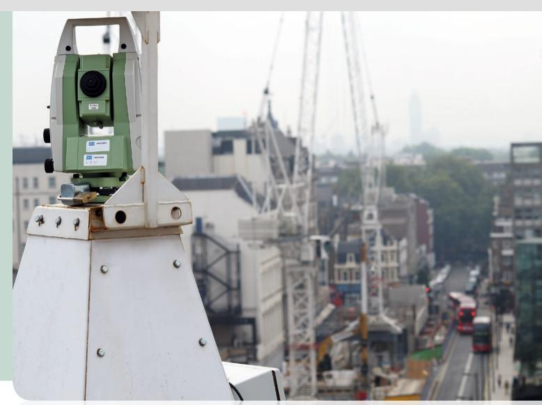
Up to 49 Leica TM30 total stations were used to monitor building movement in the surrounding Paddington Station.
