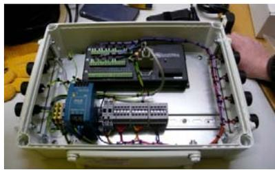
Datalogger configuration for Inclination Sensors and Anemomete
