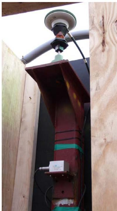
Co-located AS10 GNSS Antenna, 360 Prism° and Dual Axis Inclinometer.
