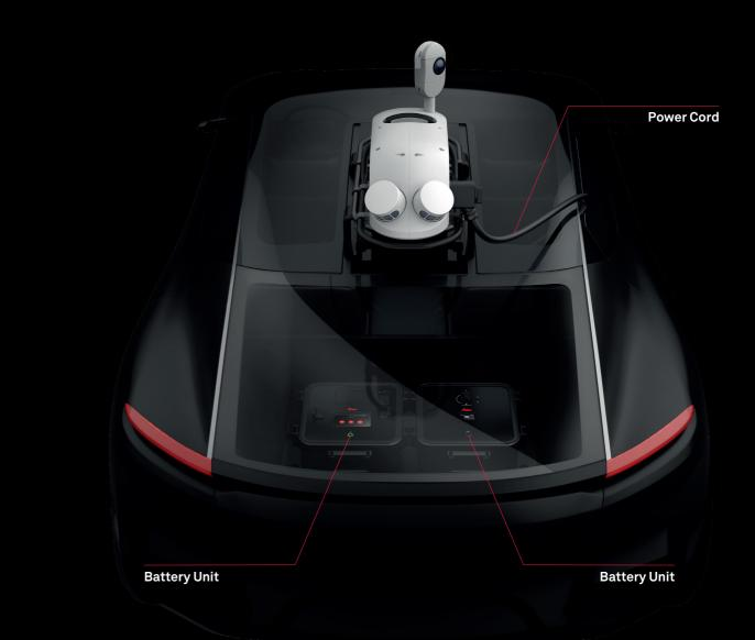
Dual scanners for when higher point cloud coverage is required, capturing 600'000 points per second.
