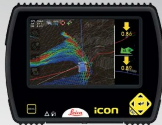
Display of the current snow depth on the machine display enables autonomous working
