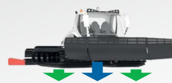
Recording of the snow depth under the snowcats or the clearing plough
