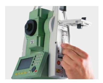
The Leica FlexLine TS06plus communication side cover enables cable-free connection to any data collector via Bluetooth®, for example the field-controllers Leica CS20 controller or Leica CS35 tablet with Captivate software. The USB-stick enables the flexible transfer of such data as GSI, DXF, ASCII, LandXML and CSV.
