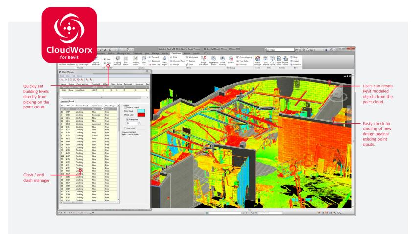
Leica CloudWorx for Revit is a breakthrough plug-in for efficiently using rich as-built point cloud data, captured by laser scanners, directly within Revit for simpler and faster BIM modeling of existing buildings. This is useful for a wide range of BIM activities including retrofit design, construction and operations, and lifecycle asset management of the building. It provides a virtual visit to the site within Revit with a complete view of the captured reality.
