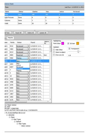
All new point cloud clash/anti-clash manager enables the user to perform interference checking against specified geometry and the point cloud.
