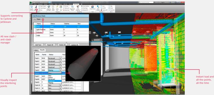
Efficient management, viewing and review of as-built laser scan data and 3D project design model for architectural, plant and civil planning and construction projects.
