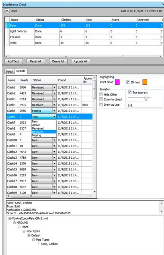
Point cloud clash/anti-clash manager enables the user to perform interference checking against specified geometry and the point cloud. Export clash manager results for easy reporting or analysis.
