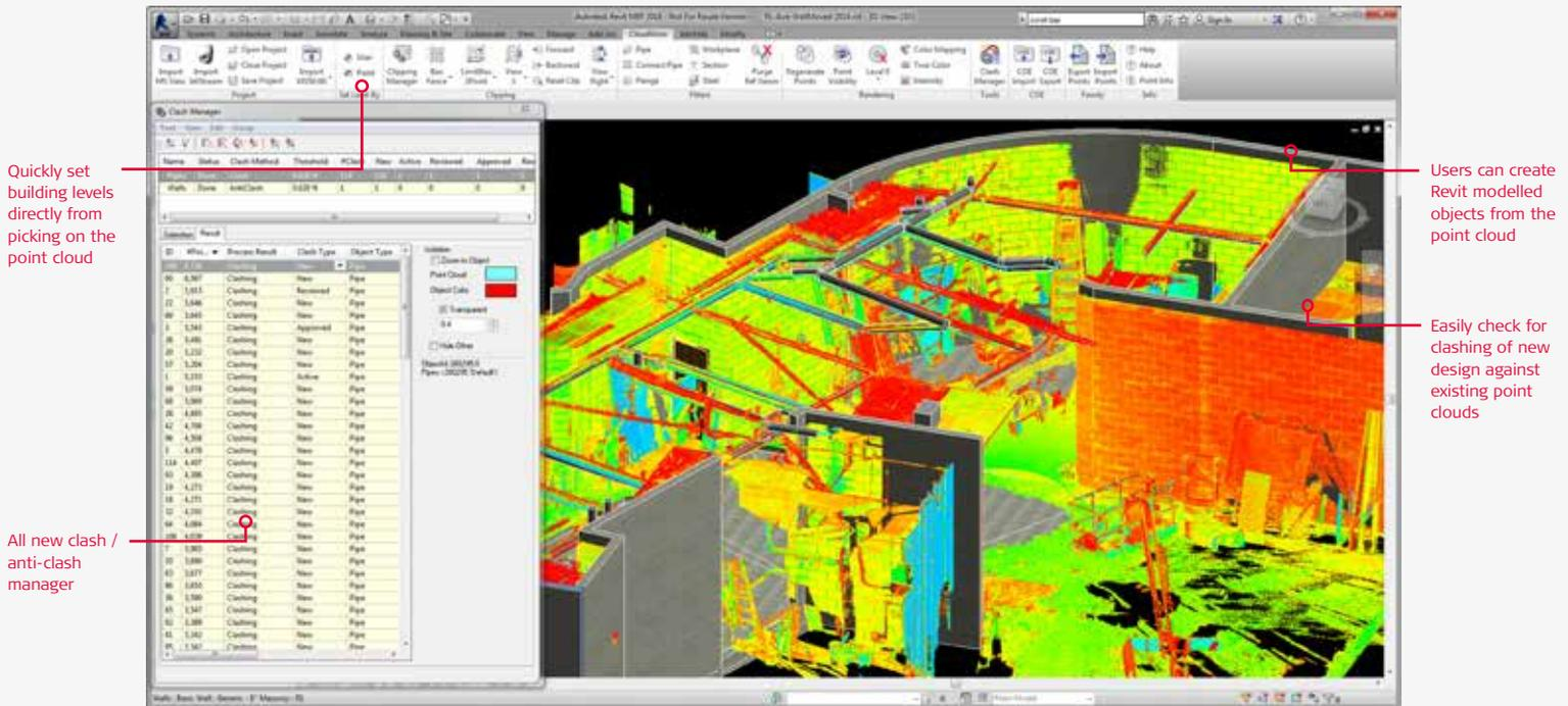
Leica CloudWorx for Revit is a breakthrough plug-in for efficiently using rich as-built point cloud data, captured by laser scanners, directly within Revit for better BIM modelling of existing buildings. This is useful for a wide range of BIM activities including retrofit design, construction and operations, and lifecycle asset management of the building. It provides a virtual visit to the site within Revit with a complete view of the captured reality.
