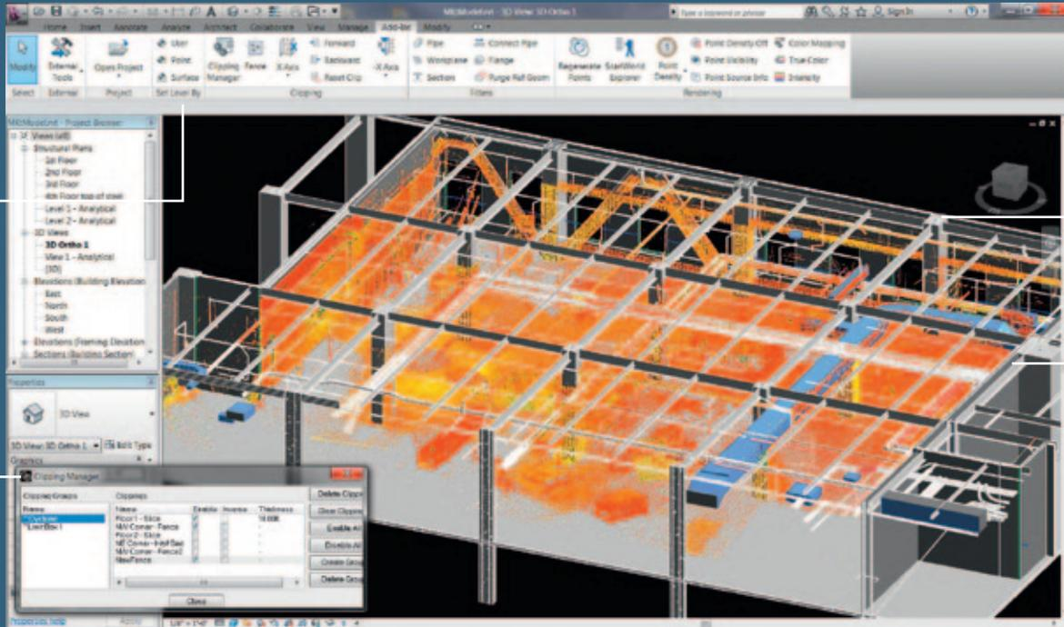
Quickly set building levels directly from picking on the point cloud.
