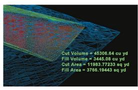
Ground surface TINs and other meshes are easily created and offer great value. Here is an automated report analysing cut and fill quantities using before-and-after scan data of a ground surface.
