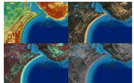
Point cloud in elevation, RGB, CIR and NIR view
