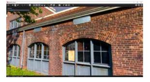
The easy-to-use JetStream Viewer allows for 3D navigation (with support for 3D mouse), visualization with HDR image support, measurement, image and video screen capture, quick limit boxes, and, when connected to the JetStream Enterprise server, access to saved UCS' and limit boxes/slices.
