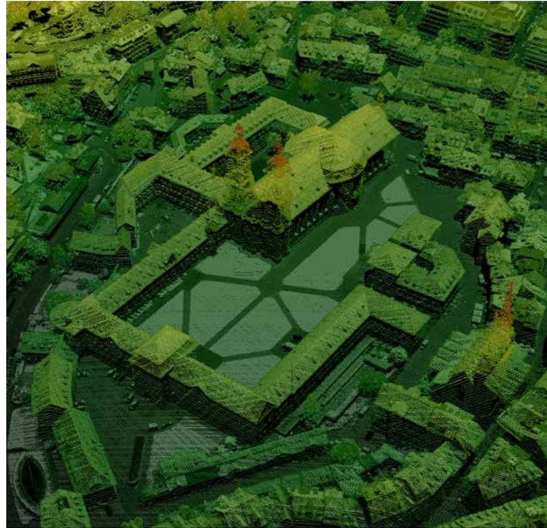
Fig. 7: Cathedral, St. Gallen, CH, acquired from 1000 m AGL at 130 knots & 40° FOV; 25 points/m<sup>2</sup>
