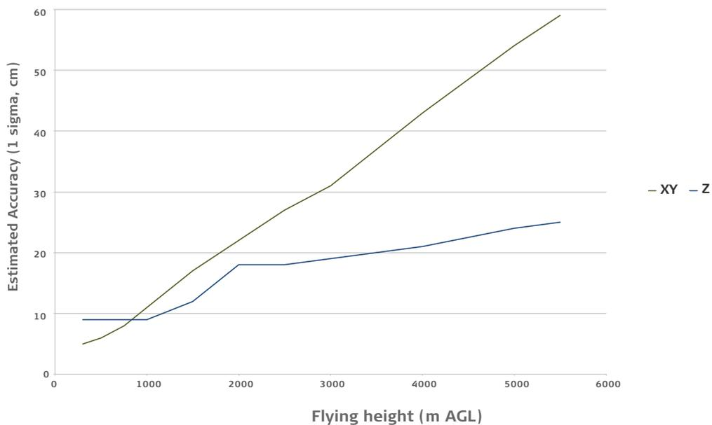
Fig. 5: Estimated accuracy (system level, including GNSS/IMU error).
