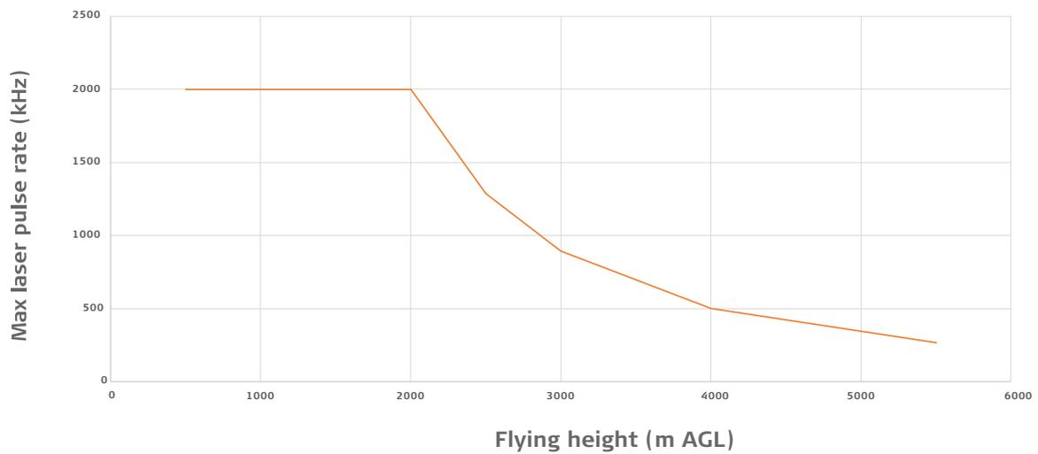
Fig. 4: Performance envelope for specified detection limit. Note: higher accuracy obtained at lower pulse rates for any given flight height.
