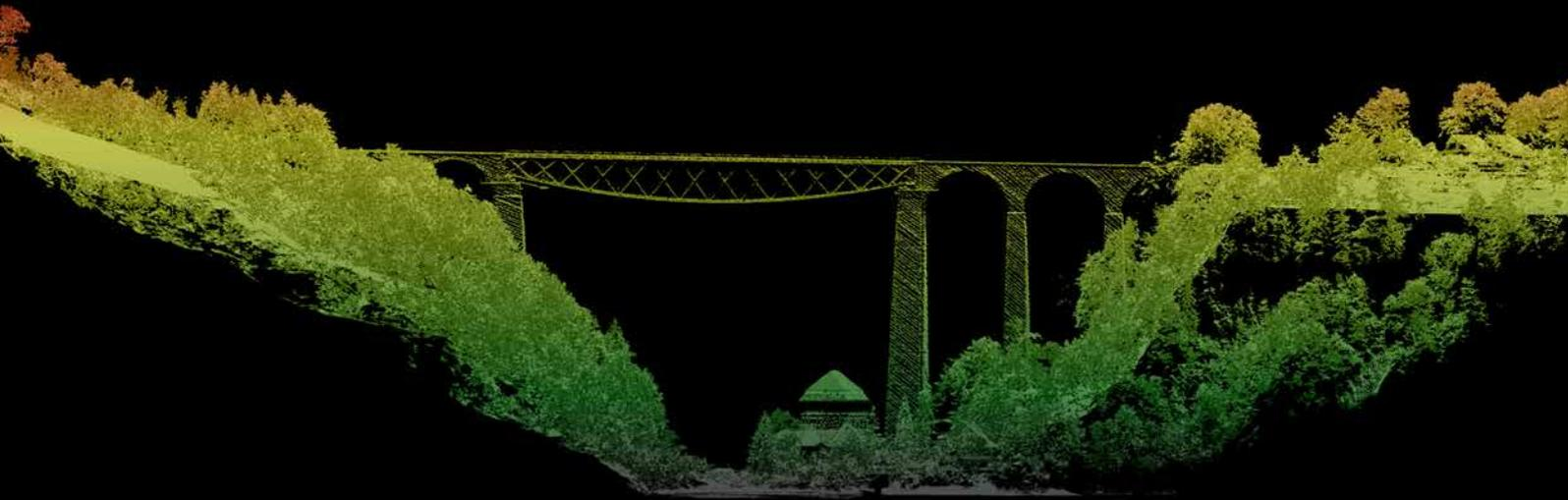
Fig. 1: Bridge and Ravine, St. Gallen, CH, acquired from 1000 m AGL at 130 knots & 20° FOV; 50 points/m<sup>2</sup>
