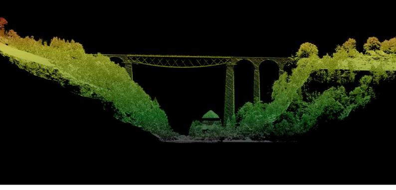
Fig. 1: Bridge and Ravine, St. Gallen, CH, acquired from 1000 m AGL at 130 knots & 20° FOV; 50 points/m<sup>2</sup>
