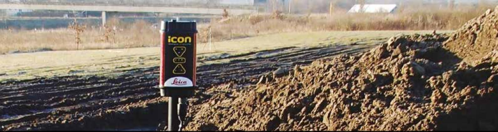
The system can be mounted on a broad range of machinery such as scrapers, dozers and agricultural tractors, automatically controlling and adjusting the work.
