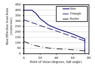
The scan rate (cycle rate in Hz) is user-selectable from 0 to 200 Hz (depending on scan pattern selected) in 0.1 Hz increments via the graphical user interface. System control software prevents out-of-range inputs for scan rate based on user selection for FOV and scan pattern.
