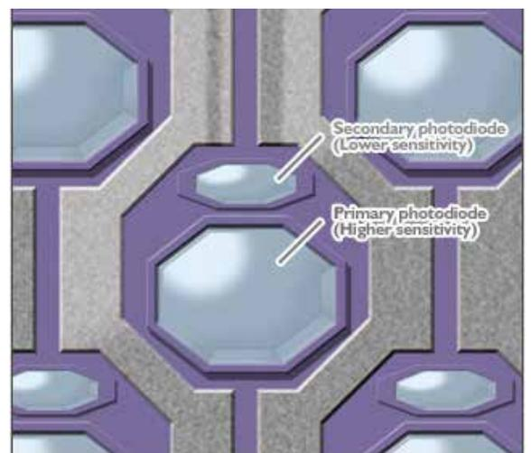
Figure 3: Example HDR Imager: Fuji SuperCCD high dynamic range image sensor [3].
