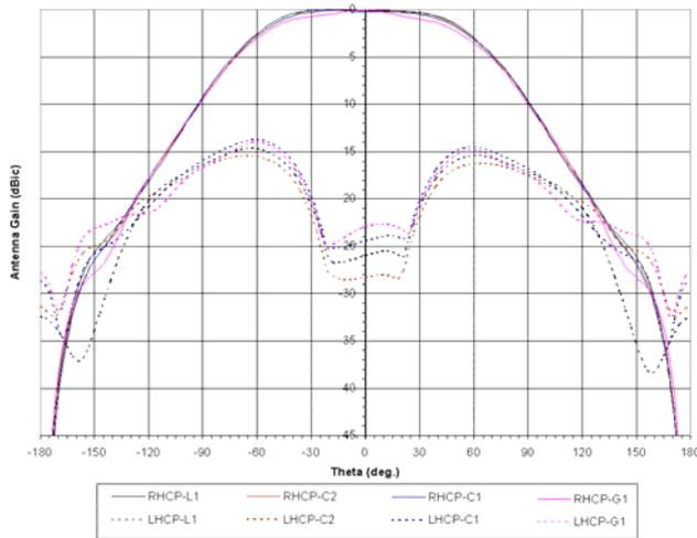
Figure 4: High-band antenna radiation pattern for AR25
