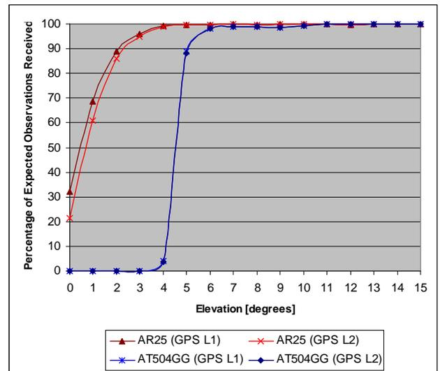
Figure 6: Completeness of observations by elevation for the AR25 and the AT504GG
