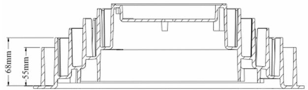
**Figure 3: Cross-section of AR25 showing the groove depths**
