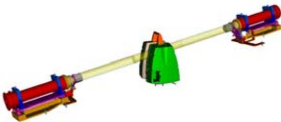
**Figure 16:** Antipodal placement of the ATEC telescopes allows the telescopes to observe their relative placement, when the scanner is removed. This is a patented twist on the idea of auto-collimation techniques that critically allows for arc second level observation and calibration of laser scanners.
