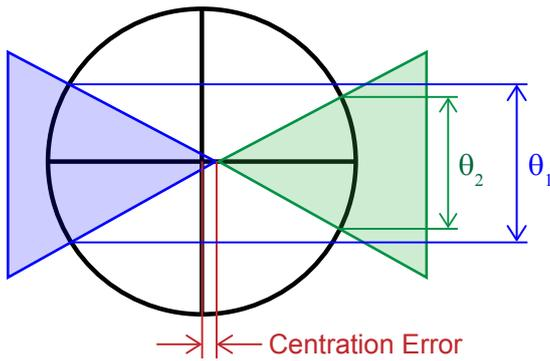
**Figure 8:** Optical encoder disk centration error causes significant error. Leica Geosystems manufactures each of the optical encoders and mounts them using a special fixture with a microscope and gentle striker. The unit is rotated slowly before the glue dries and adjusted by hand with the impact striker to minimise centration error.
