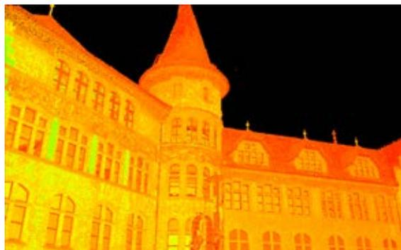
**Figure 2:** Laser scan of a building provides a lot of detail. Literally this view shows in context millions of measurements; together, they look like a photograph.
