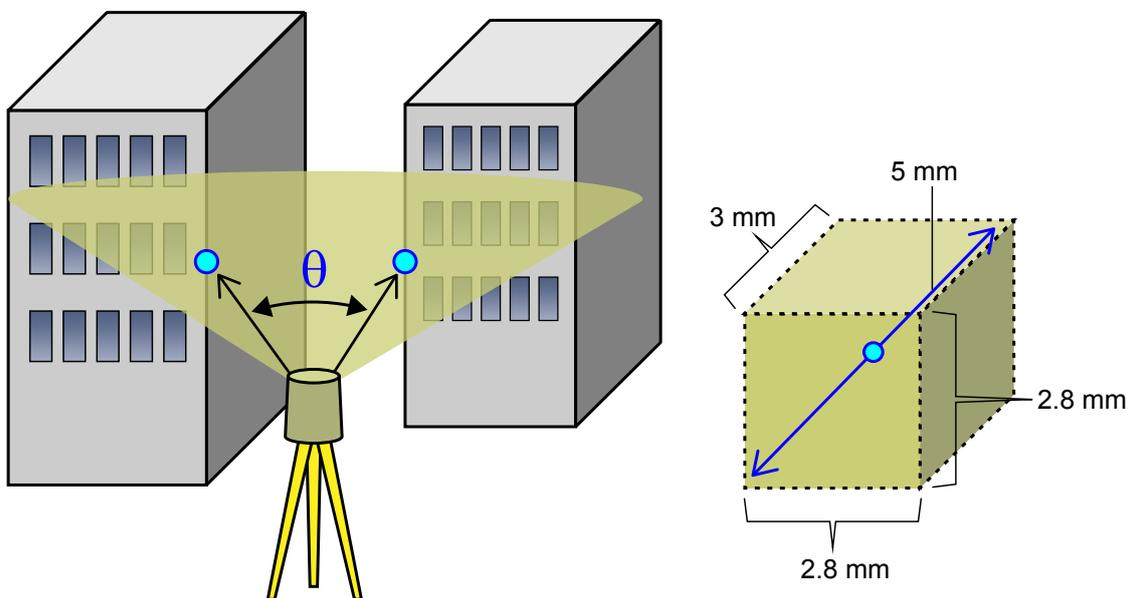
**Figure 7:** Measuring the space between two buildings. The diagonal one sigma error is swiftly computed from the specifications and the measurement situation. Without the angular accuracy specification there is no way to compute the error bound.
