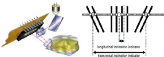
**Figure 17:** Leica Geosystems tilt sensors are also based on using a small line camera, much like the angular encoders. Much like the angular encoders, their sensitivity is very high, less than 1 arc second.
