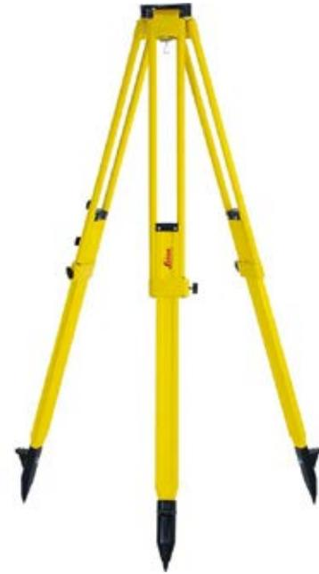
**Figure 4:** Leica Geosystems surveying tripods are carefully engineered, but are not infinitely stiff. Neither is the ground on which they are placed, in the real world. Notice the colour is bright, which makes it easy to spot but also more subtly reflects instead of absorbs sunlight, instead of, say, black. Notice also the little foot pads at each tripod foot – you step on those to firmly set the tripod. No stomping your feet.
