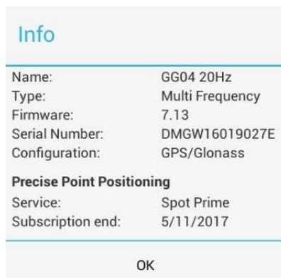
Figure 5 - GG04 smart antenna settings in Zeno Connect PPP service license details
