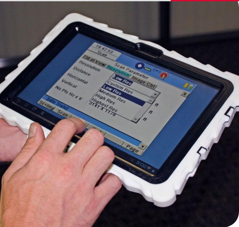
■ **Operating the Leica ScanStation via tablet.**
