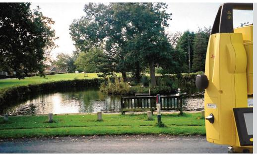
The reflectorless capability of the Leica Builder was particularly useful to measure the detail of the island in the middle of the small village pond.
