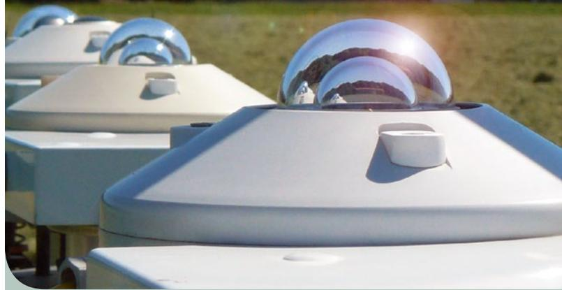
■ vTI also uses sensors to measure global radiation.
