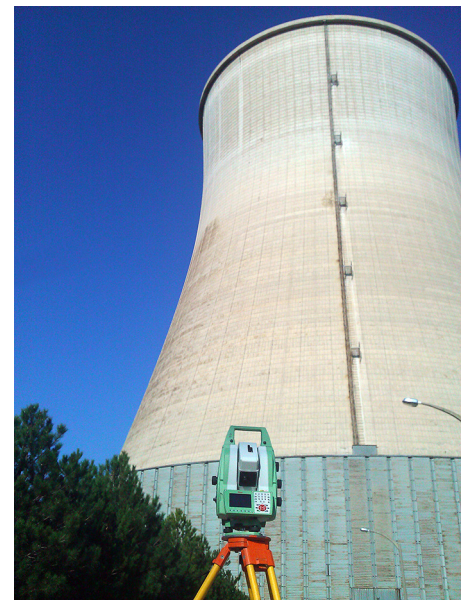
Scanning at distances of up to 300 m.
