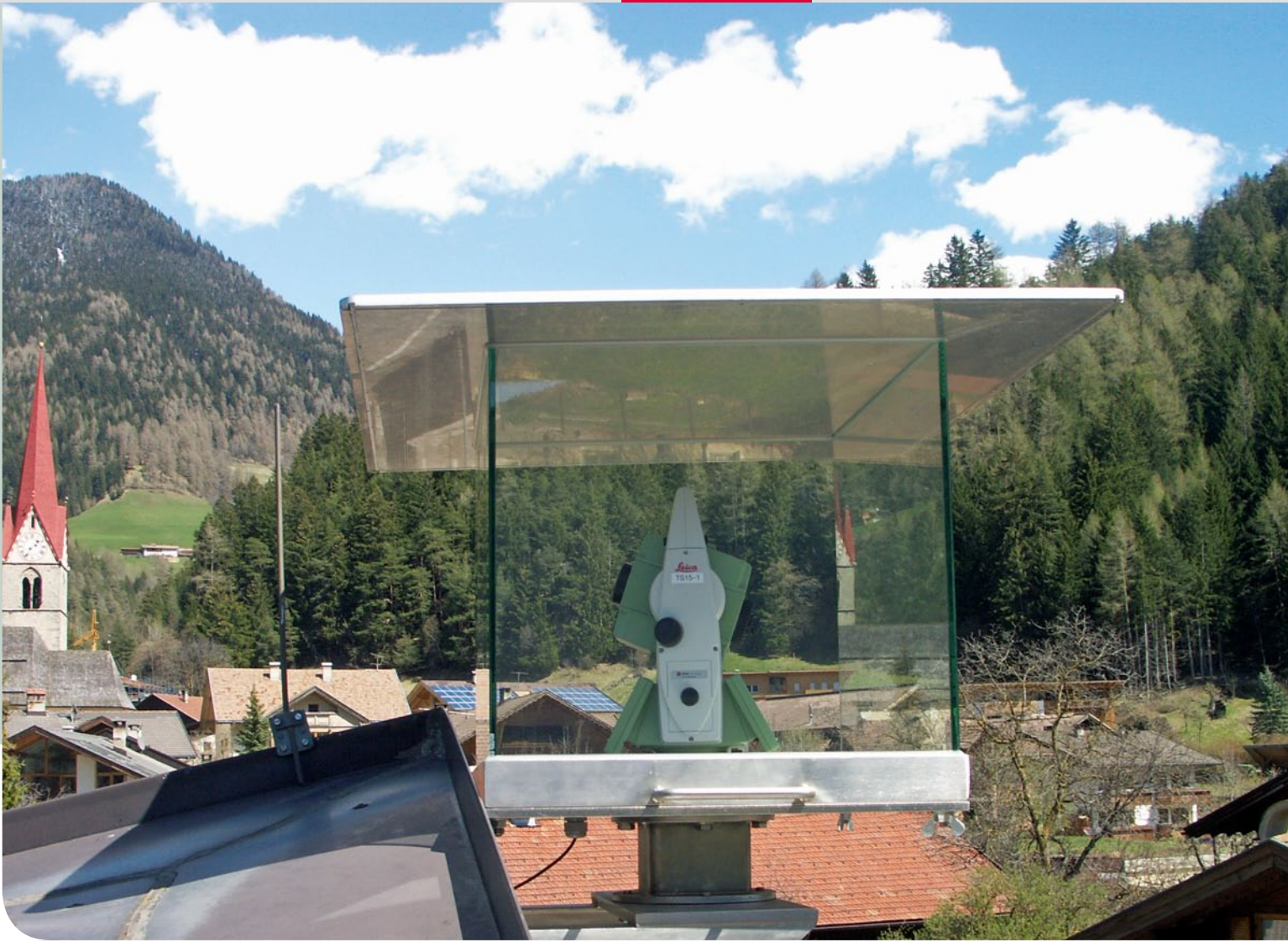
■ A Leica Viva TS15 Total Station monitoring surface movements in Mals.
