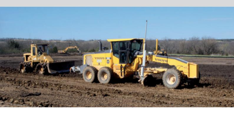
file from the engineer, and my son converts that to a usable 3D model - a Digital Terrain Model. That model is on a flash card and we install it into our two dozers, the finish motor grader and the rover."
