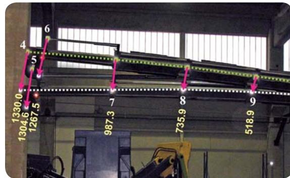
■ The movements of the crane's arm were measured with a Leica TS30.
