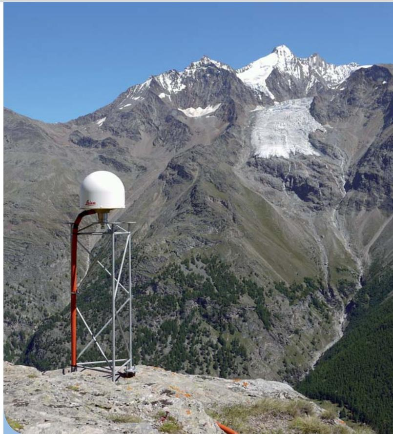
■ Reference station on a swisstopo trig point above the Randa avalanche zone (Wallis Canton, CH). The Dirru block glacier can be seen on the opposite side of the valley.
