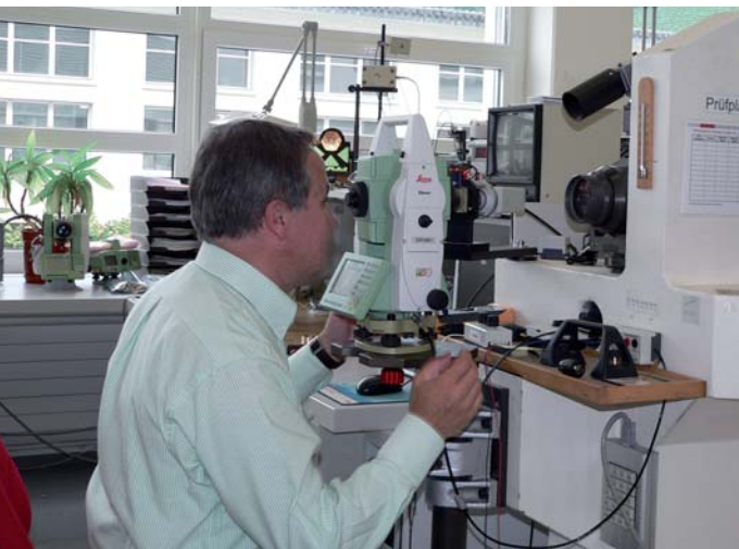
■ CTS staff member Guido Grossmann adjusting a Leica TCP1205+ total station.
