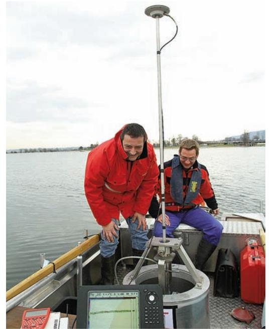
**"The measuring points are displayed in the Leica MobileMatriX in real time, thereby enabling an intelligent sequencing of the measurements and renders costly new measurements unnecessary, which saves our crew much time and guarantees exact data gathering."**
