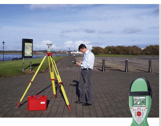
The project was to create a system for the collection and storage of asset inventory data based upon ESRI ArcGIS and the Leica Zeno 15 GIS handheld, and evaluate with respect to ease of use and geospatial accuracy.
