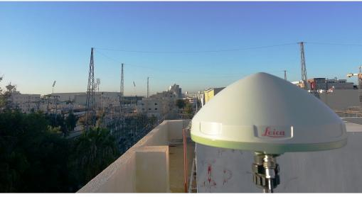
Leica GR10 receivers and AR10 reference antennas deliver RTK correction data for the precise positioning of IDECO's electrical assets.
