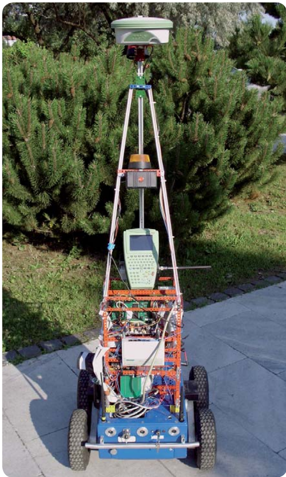
■ Outdoor mobile robot with Leica GPS1200.
