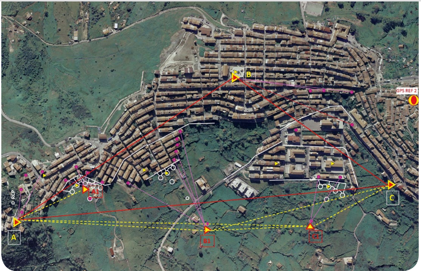
■ Monitoring network with GPS baselines (red and yellow lines) and total station observations (pink lines).
