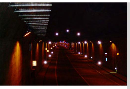
The tunnels of the M-111 road, to its passage under the runway of Madrid - Barajas airport, must be monitored for deformation of the prefabricated structure. The monitoring is necessary because of the weight of 20 meters of ground and other materials that must be supported, in addition to the transit of airplanes.
