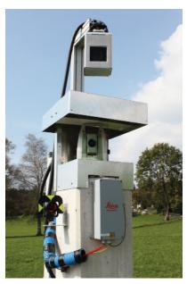
Measurement pillar with Leica TM30 and webcam
