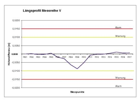
The graph shows the longitudinal profile with the measurement series V prisms. The measurements from P506 to P511 clearly show the formation of the sag in the track.
