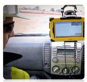
Height check: Leica iCON CC60 in the pick-up.
