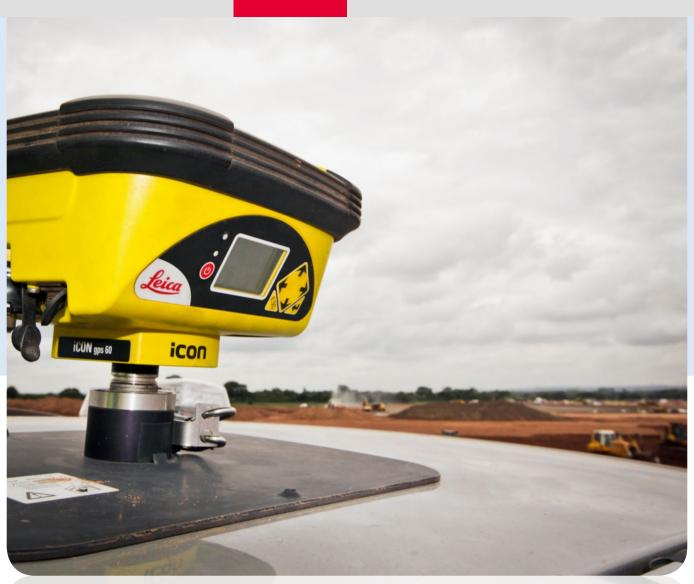
■ Leica iCON GPS 60 on the roof of the pick-up: the project manager can drive around the site, checking heights.
