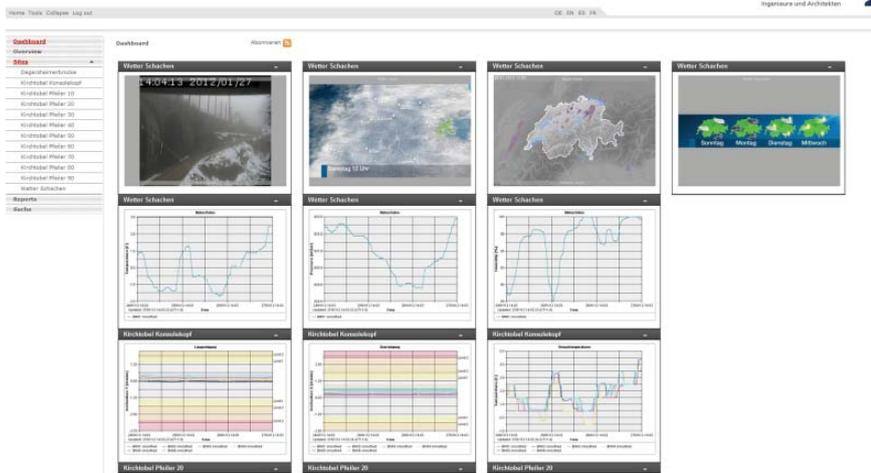
Graphical visualisation of the monitoring data in Leica GeoMoS Web: web cam image, weather forecast, rain radar, meteo data, inclinations with shown limit levels, etc.
